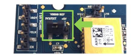
6. Plug the GYPRO<sup>®</sup> or AXO<sup>®</sup> Evaluation Board on the Arduino Board, using the 5 connectors supplied by Tronics. **The correct position is to have the Arduino board on top (above the Evaluation board).**
